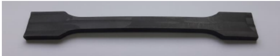
Figure 6 The test piece made of plastic, which was subjected to a strength analysis
